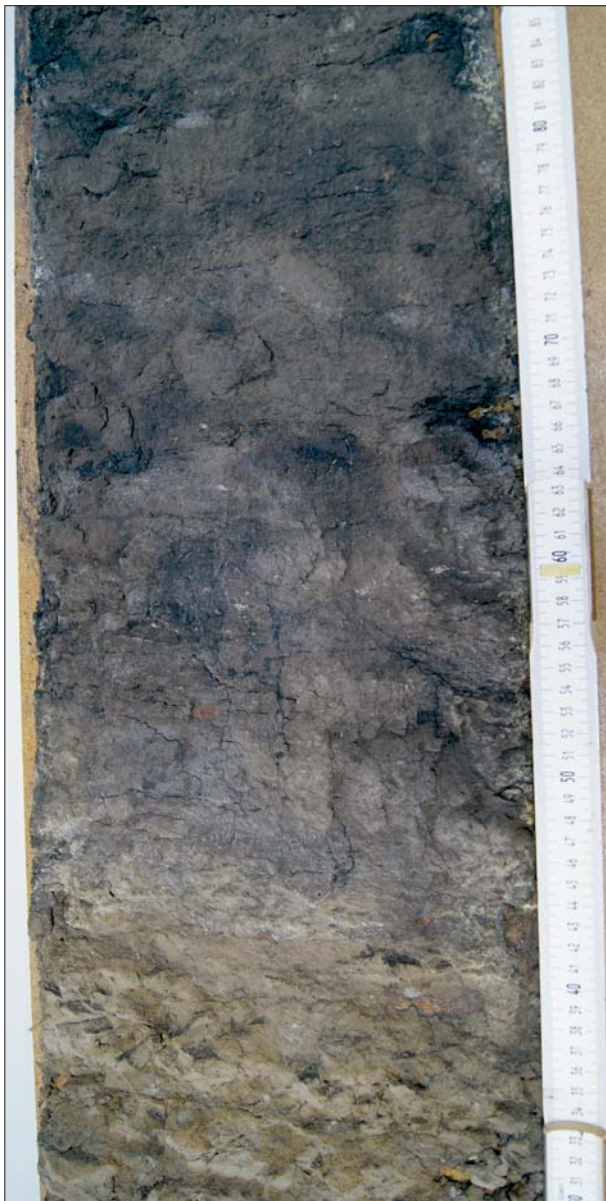
Fig. 7 Photo taken from soil monolith of the upper parts of profile Schöningen 12 B (92) in organic richer facies. – (Photo B. Urban).
